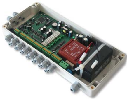
Figure 4. The DOX access controller.
