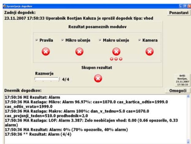
Figure 3. The graphical user interface of our intelligent access control system for an irregular access. The four big circles represent classifications of the four stand-alone modules. The single circle bellow represents the joint and final classification, while the text at the bottom shows the explanations for each module.
