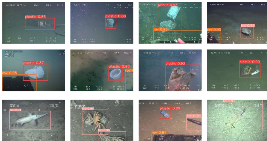
Figure 14: Plot of results of detection in different underwater scenarios. The trained model is used in different detection scenarios and different detection objects for detection and the results are shown in Fig. The results show that our model has strong generalization ability in underwater detection sites.
