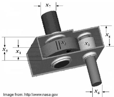
Figure 3: Speed Reducer.
