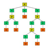
Figure 7: Example of a production plan (P) defined by ontology, where some production steps (S) have an operation (O) associated and some have another production plan associated.
