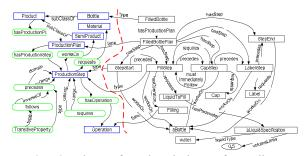
Figure 3: Ontology for description of a discrete production process as a series of consecutive/parallel production steps in which particular manufacturing operations are executed upon the semi-product; right hand side shows sample plan describing production of a filled bottle.
