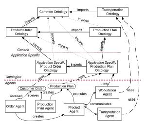
Figure 1: The upper part shows modularized manufacturing ontology with generic and application specific parts including *import* relation between individual ontology modules; the dashed *import* lines show transitive closure of the *import* relation. The lower part shows agents that use different modules of the ontology.
