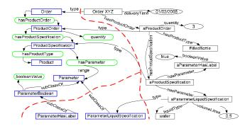
Figure 2: Schema of the ontology for customer order specification (on the left); domain specific extension of the ontology for hypothetical production of a filled bottle (on the bottom); knowledge base corresponding to sample order of three filled bottles (on the right).
