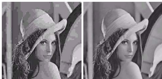
(a) JPEG compressed image, Bit rate = 0.18bpp, PSNR = 28.07 (b) TCVQ compressed image, Bit rate = 0.18bpp, PSNR = 29.24
