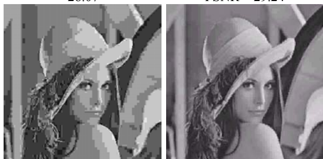
(c) JPEG compressed image, Bit rate = 0.14bpp, PSNR = 24.89 (d) TCVQ compressed image, Bit rate = 0.14bpp, PSNR = 28.41
