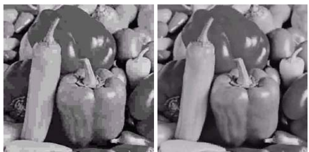
(a) JPEG compressed image, Bit rate = 0.18bpp, PSNR = 28.70 (b) TCVQ compressed image, Bit rate = 0.18bpp, PSNR = 29.40
