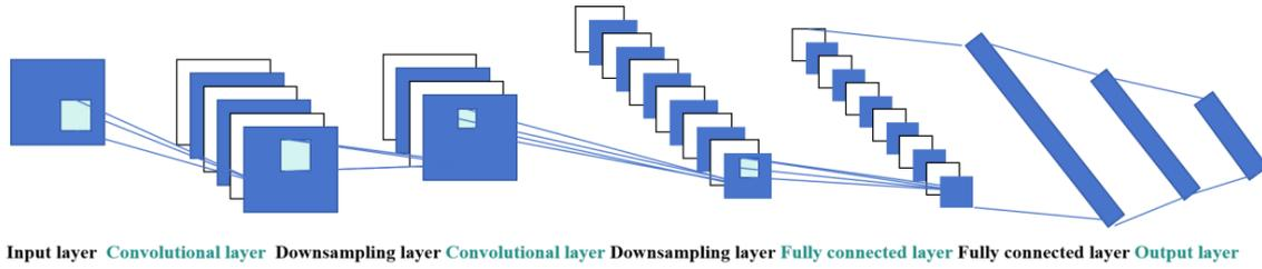
Figure 1: A diagram of the convolutional neural network
