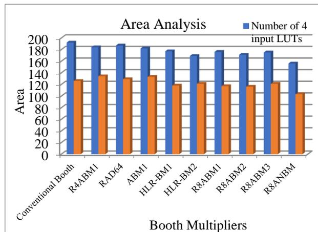
Figure 6: Area analysis of approximate booth multipliers. Area of the proposed radix-8 approximate multiplier using novel booth encoder is compared with the existing booth multipliers and it is shown in Figure 3. From the comparison chart, it is observed that, the proposed ANBE reduced the area over their existing multiplier designs. The proposed R8ANBE reduced the number of 4 input LUTs by 23.07%, 17.94%, 19.87%, 16.66%, 13.46%, 8.33%, 12.82%, 9.61%, 12.17% and number of
