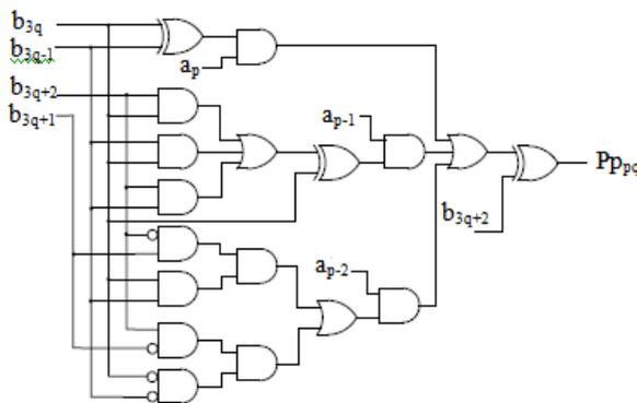
Figure 2: Logic diagram of existing R8ABE1
