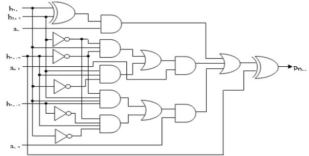
Figure 3: Logic diagram of the proposed ANBE
