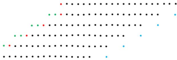
Figure 4: Dot diagram of proposed Radix-8 approximate novel booth multiplier
