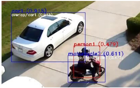
Figure 2: Results applying IoU; the Bounding Box of "person1" is overlapping the Bounding Box of "motorcycle2."
