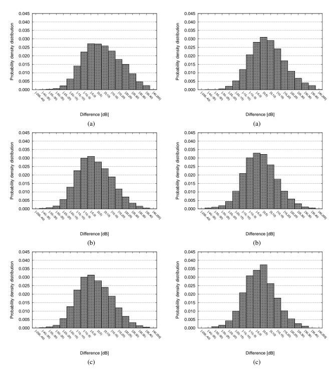
Figure 2: Probability-density distribution of radio predictions against the field measurements of network Net<sub>1</sub> over a rural area using the: (a) manually-calculated parameters, (b) analytically-calculated parameters, and (c) optimized parameters.
