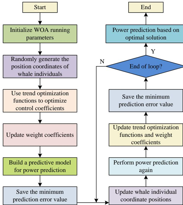
Figure 3: Wind and solar power prediction process based on NDO-WOA
