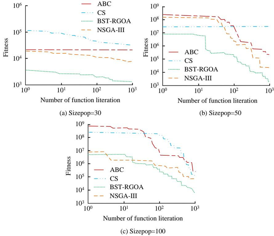
Figure 9: Convergence curves of various algorithms under different population sizes
