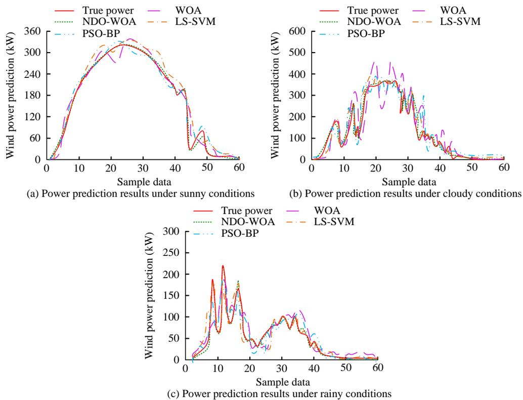
Figure 7: Power prediction results of various algorithms under different meteorological conditions
