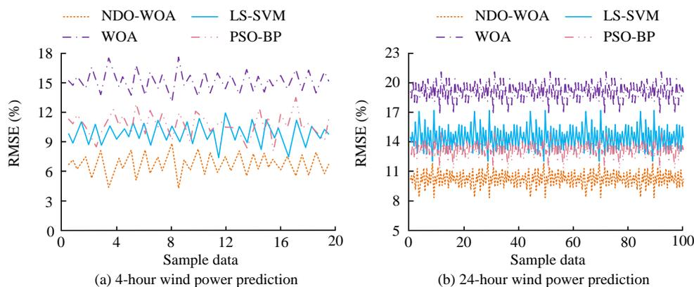
Figure 6: RMSE values for power prediction of various models at different time scales
