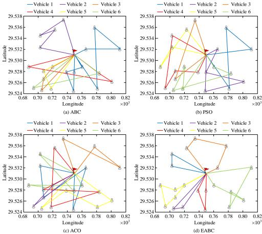
Figure 10: Optimal path planning diagrams for different algorithms.
