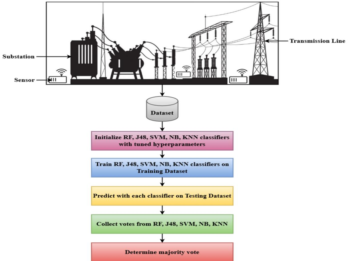
Figure 1: System architecture of SPHC algorithm
