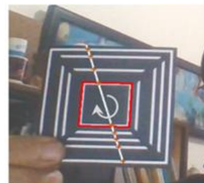
(b) Real OILU markers identification based on cross ratios computation
