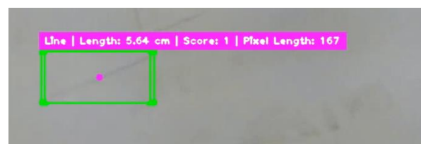
Figure 16: Bounding box display showing maximum length
