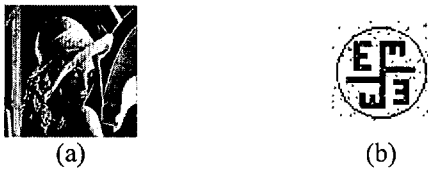
Figure 12: Robustness test against image rescaling (2:1) for VSSW: (a) rescaled image; (b) extracted watermark.
