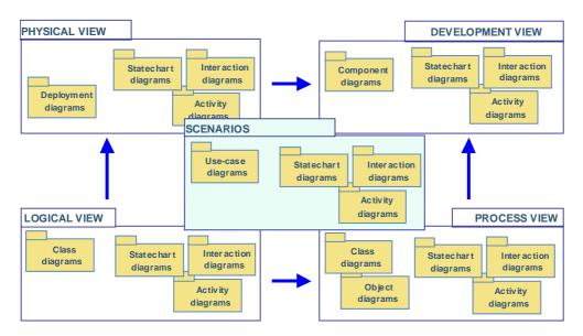
Figure 1: The "4+1 view model and its mapping to UML diagrams.
