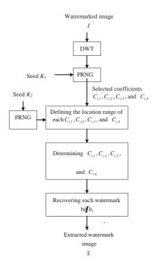
Figure 4: Block diagram of the proposed watermark extraction process.
