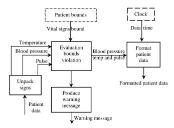
Figure 2: Partial Data Flow Diagram of SA
