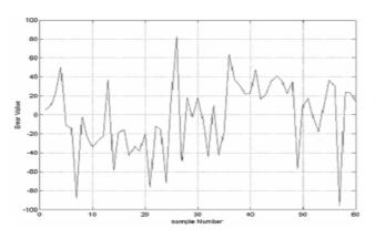
Figure 9: Error between Actual and Predicted Data ARMAX Model.
