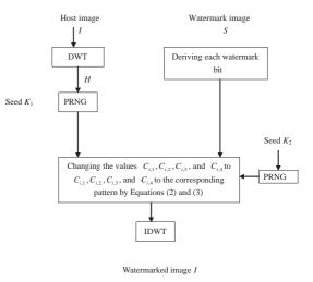
Figure 2: Block diagram of the proposed watermark embedding process.
