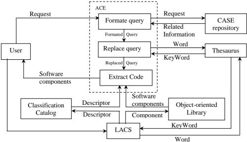
Figure 5: Data Flow Diagram of CART
