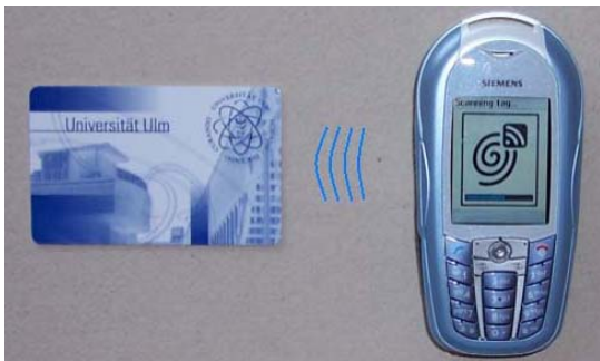
Figure 1: Student ID card of Ulm University, and prototype phone equipped with RFID communication hardware.
