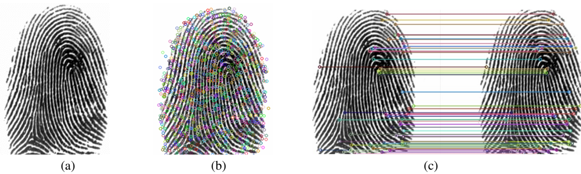
Figure 1: Fingerprint local feature extraction and matching: (a) Raw fingerprint image, (b) Extracted local features using the SURF detector, and (c) Fingerprint matching using the extracted local features. The number of matched features have been reduced for a clear representation purpose.
