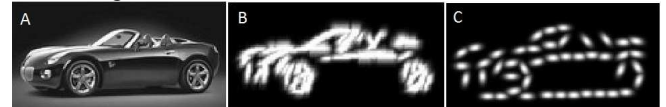
Figure 3: Edge detection using Gabor wavelets, A. Original image[1], B. edge detected image with a large number of features without sparsity, C. edge detected image with a small number of features where sparsity is enforced.
