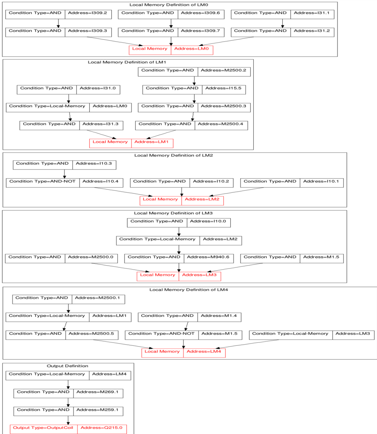
Figure 7: The state-based graphical representation of the rung logic corresponding to the first Output Coil instruction.
