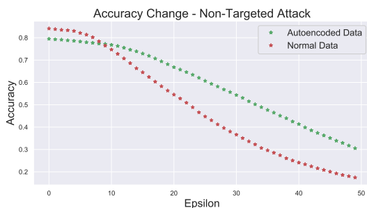
Figure 103: Comparison of accuracy with and without denoising autoencoder for non-targeted attack and Fashion MNIST Dataset
