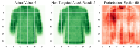
Figure 76: Value change and perturbation of a non-targeted attack on model without autoencoder for Fashion MNIST Dataset
