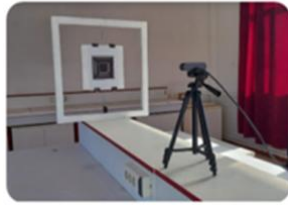
(a) A high-resolution front camera is used to record video sequences at various distances ranging from 0.2 to 4 meters
