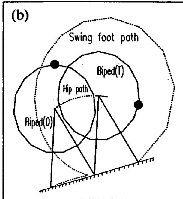
Figure 4: Feet and Hip Paths for a Single Periodic Walking Step: (a) on level ground, (b) up a  $\alpha = 15^\circ$  incline.
