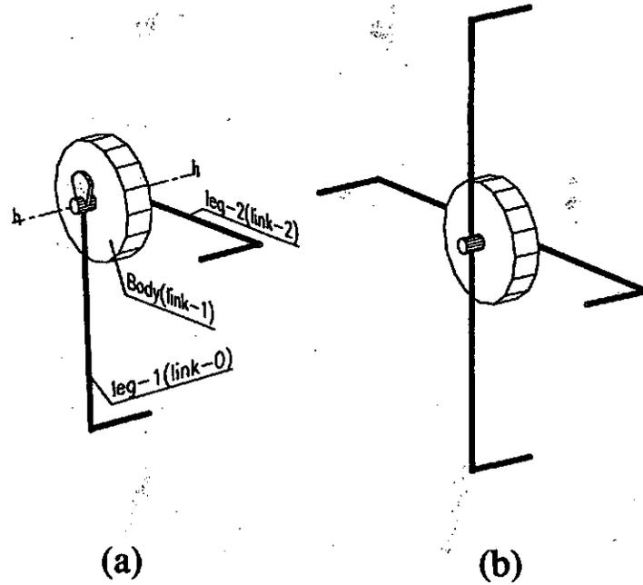
Figure 1: Biped Machines: (a)  $N_F=1$  foot per leg, and (b)  $N_F=2$  feet per leg.
