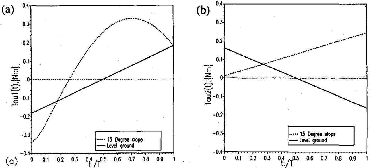
Figure 7: Joint Torque Trajectories: (a) stance leg torque  $\tau_1(t)$ , and (b) swing leg torque  $\tau_2(t)$ .
