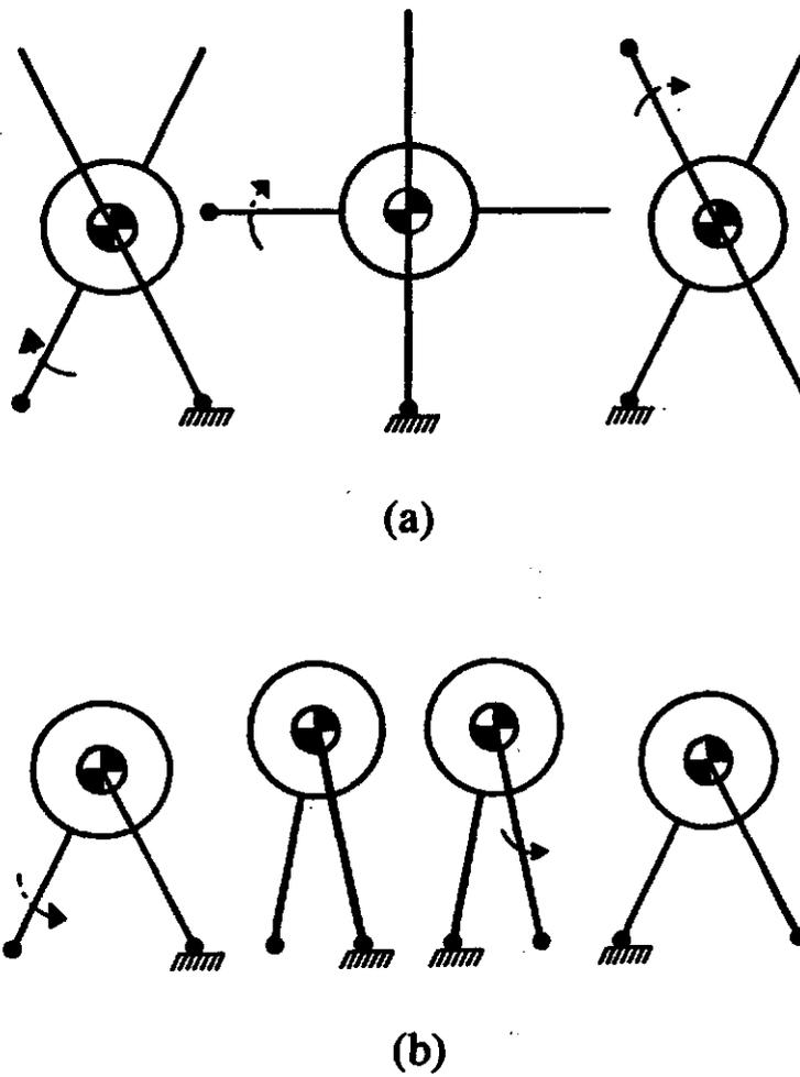
Figure 2: Walking Gaits: (a) wheel gait for biped with  $N_F=2$ , and (b) inchworm gait for biped with  $N_F=1$ .
