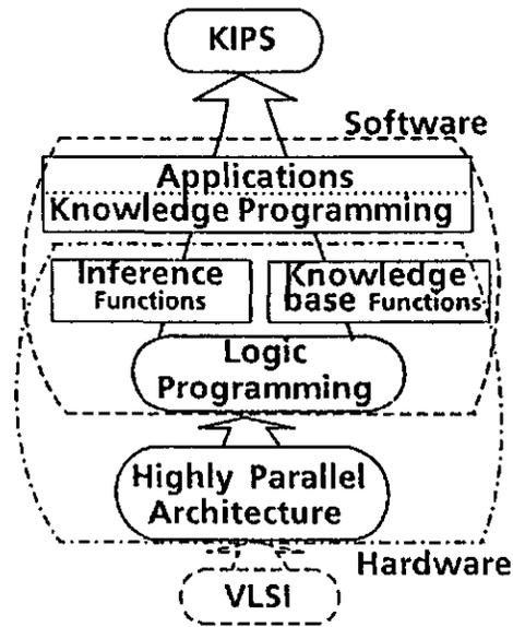
Figure 1: Concept of the Fifth Generation Computer
