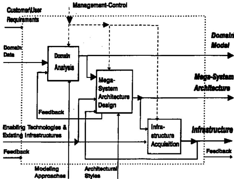
Figure 2: A Process Diagram for the Mega-System Task
