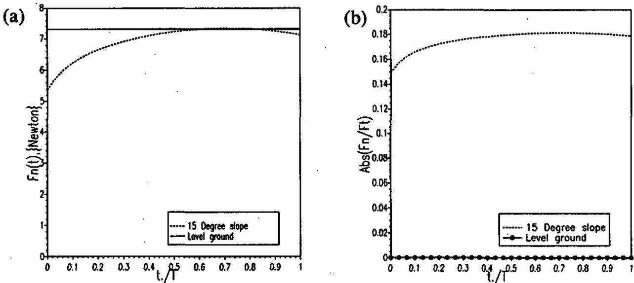
Figure 5: Foot Force Trajectories: (a) normal force  $F_n(t)$ , (b) required friction coefficient  $\mu(t) = |F_t|/F_n$
