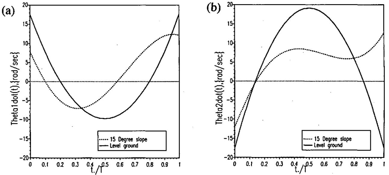
Figure 6: Joint Velocity Trajectories: (a) stance leg hip joint velocity  $\theta_1(t)$ , (b) swing leg hip joint velocity  $\theta_2(t)$ .
