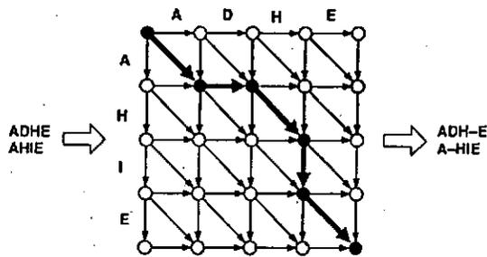
Figure 5: Two Dimensional DP Matching for Shortest Path Finding
