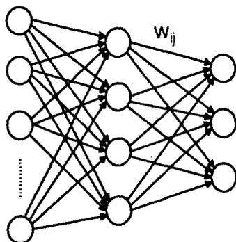
Figure 1. Structure of a feed-forward network.
